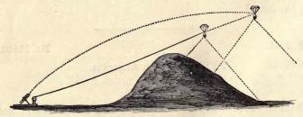
explodes, thereby liberating the camera and parachute, which may be drawn back by a cord after the exposure of the negative.
